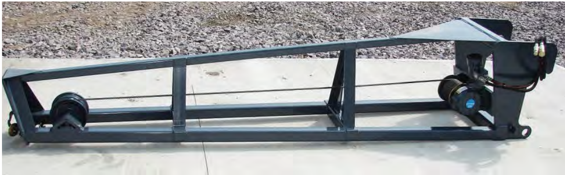
Figure 19 - Jib With Integral Winch
