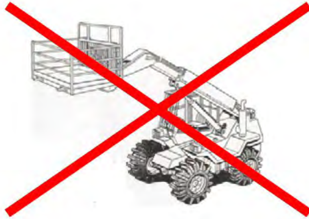
Figure 21 - Non-integrated Work Platform
